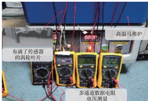
图4 将延长线连接到炉外的万用表对多组传感器的热电阻和热电压进行数据采集与测量 Fig.4 Connecting extension wire to multi-meter outside furnace and collecting measured data of thermal resistance and thermal voltage of sensors
